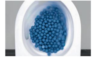
required by standard testing (DIN EN 997-2018). Flush performance is up to 10 times better than
