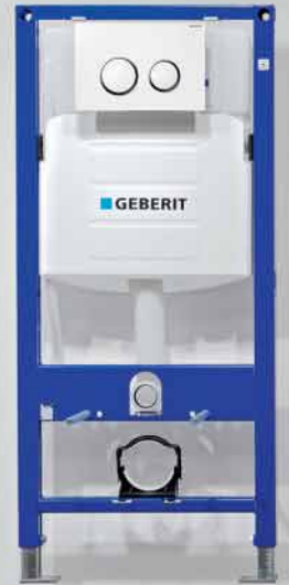
Duofix frame with concealed cistern and Sigma20 dual-flush actuator plate Tool-free installation, water-saving dual flush system for flexible application
