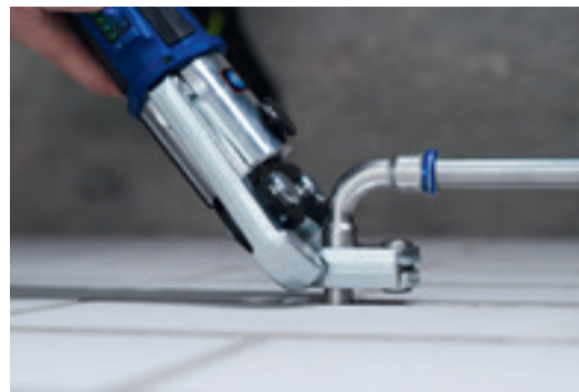
↑ For Geberit Mapress up to d35, pressing rings and adapter jaws are ideal for use in confined spaces. The compact pressing ring is positioned and securely pressed using the pressing jaw, which can swivel up to 180°.
